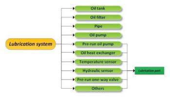
Fig. 6. Unit structure of a lubrication system
