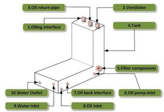
Fig. 4. Simple structure of an oil tank
